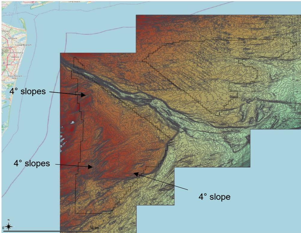
**Figure 24. Example of Slope Analysis across Hudson North and Hudson South Pilot Areas**
