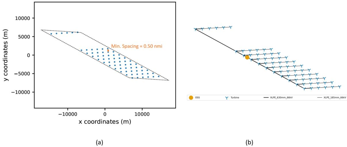
Note: Array cables are connected in series with a minimum separation distance of 65.6 ft (20 m). This distance is below the scale of Figures 6 - 12. The turbine rotor diameter is represented to scale with the blue dots at each turbine position in (a).
