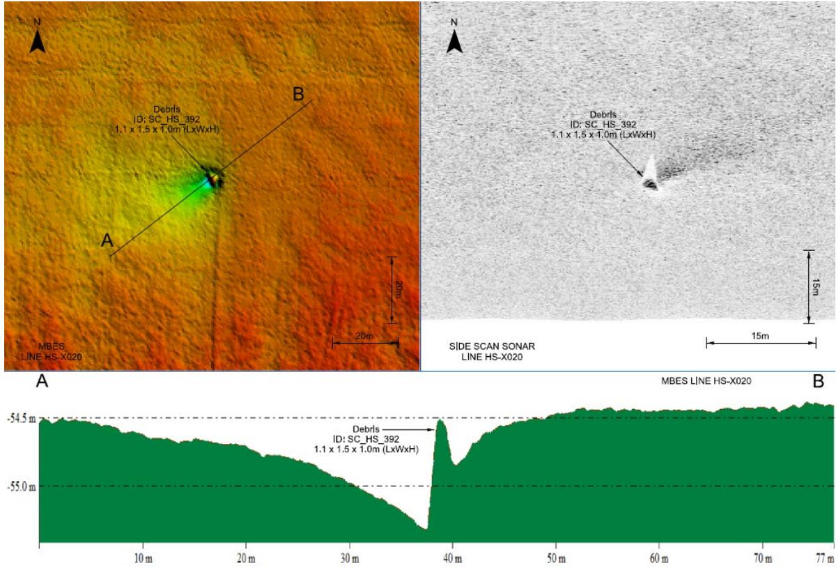
**Figure 35. Examples of Sonar Contacts with Visual Indications of Scour**
