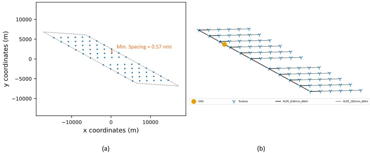
Note: Array cables are connected in series with a minimum separation distance of 65.6 ft (20 m). This distance is below the scale of Figures 6 - 12. The turbine rotor diameter is represented to scale with the blue dots at each turbine position in (a).
